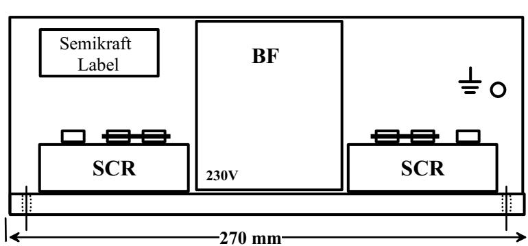
AI-L270 0,90°C/W AI-L270(F) 0,3°C/W (F) means cooled with extern Fan not in ouer delivery.
